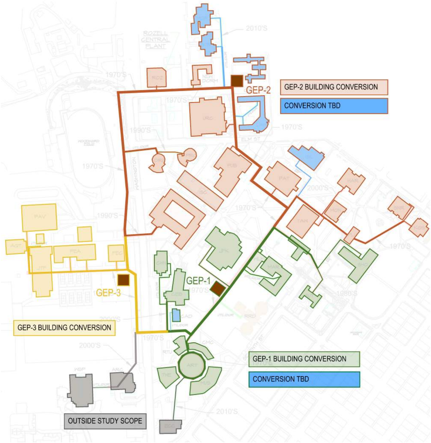
Figure 11: New Distribution Piping Deployment by Node
